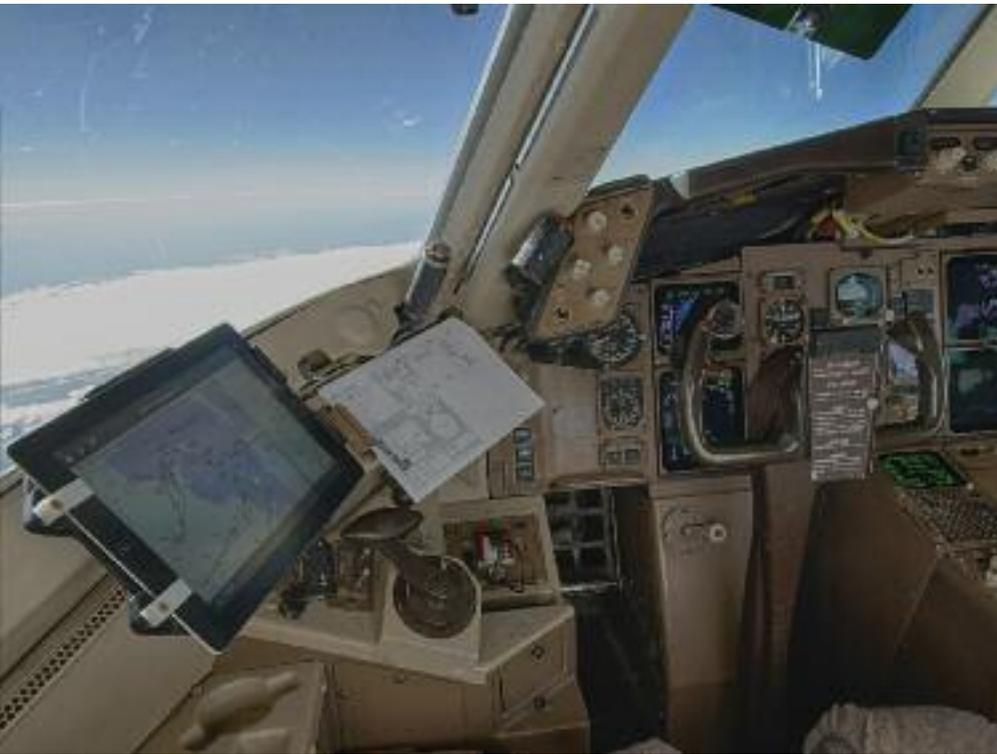
record in challenging environments,” adds Bradbury. The EFBs are not permitted for use in the take-off and landing stages. During these critical phases of flight they are kept in document stowage on the sidewall of the flightdeck. There is no data interface with aircraft systems, and the Toughbooks are not connected to back-office systems. Software is updated by engineers when necessary. easyJet issues two Toughbooks to every aircraft.
